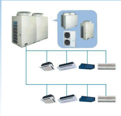
(Variable Refrigerant Systems)
